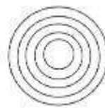
(b) Track pattern on a magnetic disk
